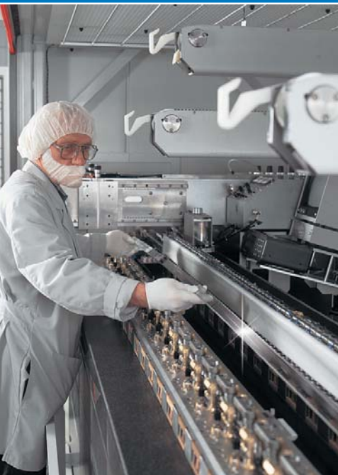
Scale-replicating equipment in a Class 100 clean room environment.
