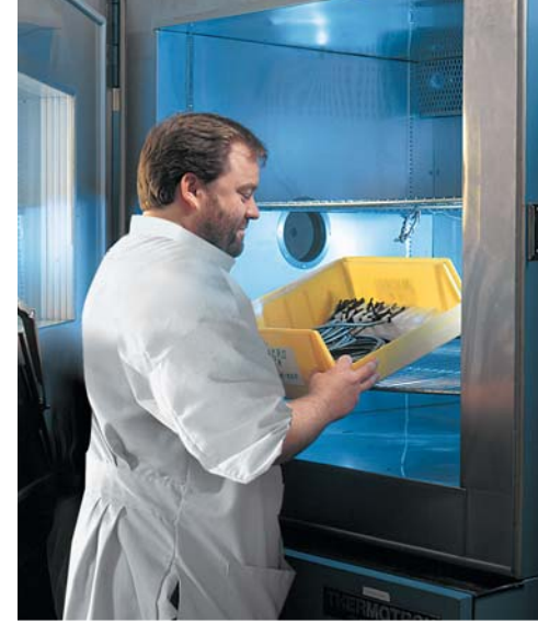
Environmental test chamber ensures that all reading heads can withstand extremes in temperature and humidity.
