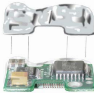
Conformal coating is applied for extra protection.
