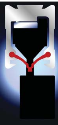
Cross-sectional view of Acu-Rite Companies Inc. precision glass scale highlighting recessed chemical resistant interlocking lipseal.
