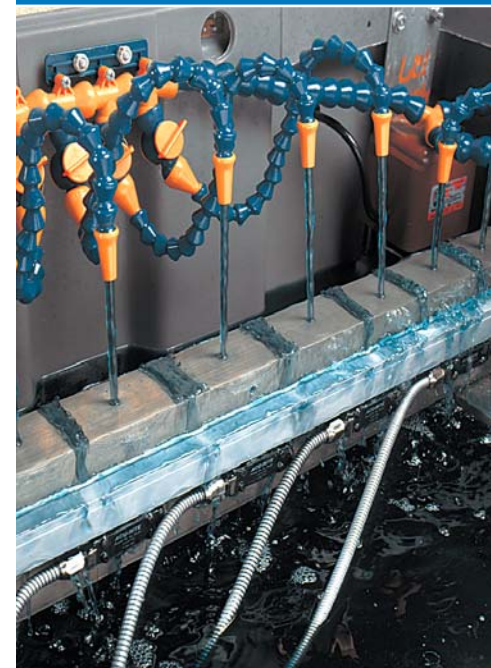
Test equipment verifies performance when subjected to flood coolant conditions.
