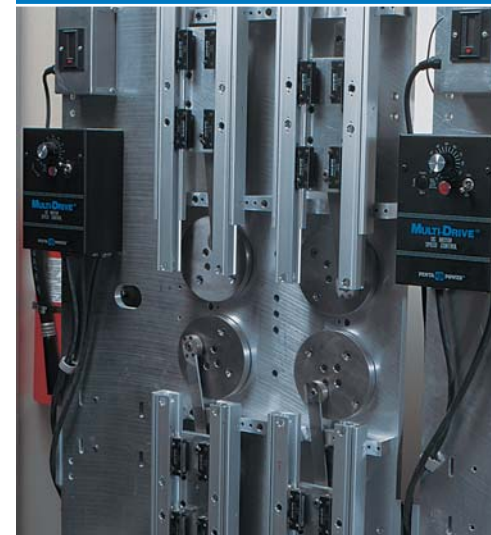
Precision glass scale test fixture verifies a minimum of 13 million cycles.
