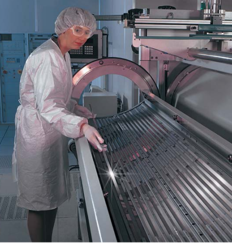
Vacuum coating equipment ensures consistent chromium deposition.
