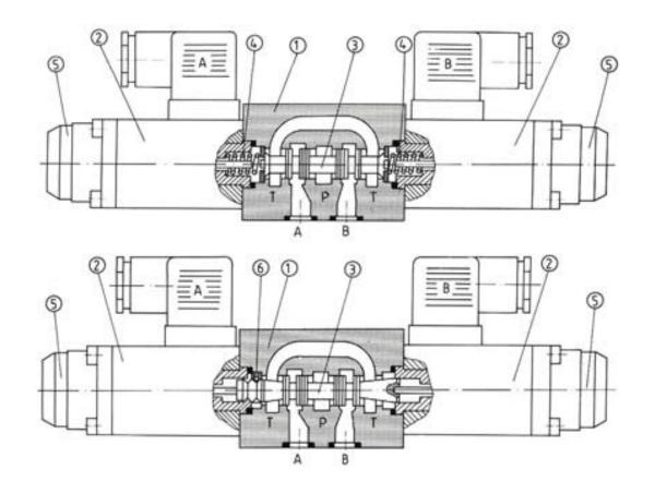
The directional valve is switched by changing the position of the spool 3 which moving along its axis separates or connects ports A, B, P or T in the housing 1. The spool is shifted by the force of the solenoids 2.
