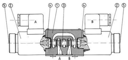
The directional valve is switched by changing the position of the spool 3 which moving along its axis separates or connects ports A, B, P or T in the housing 1. The spool is shifted by the force of the solenoids 2.
